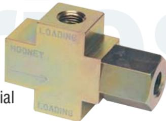
The Type 26 inspirator incorporates a special nozzle design that reduces the loading (spring case) pressure to a value below the outlet pressure allowing the valve to fully open even when the pressure differential is very small. The inspirator acts like a differential amplifier with a gain of approximately 3.
